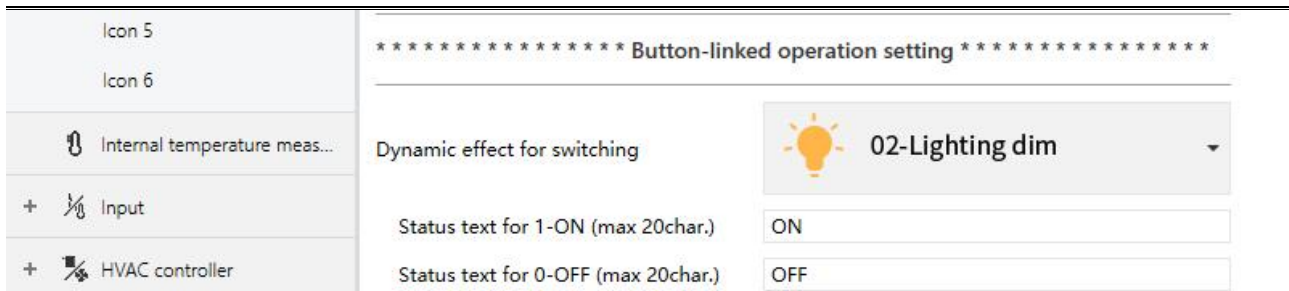
RGB / RGBW / RGBCW / Colour temperature dimming dynamic effect setting Fig.5.6.2.1 (4) Parameter setting of colour and colour temperature dimming function
